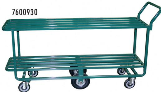
7600930 Two deck stock truck 60" x 18" with 1" sq. tubing -green, with 6 wheels - 18" spacing between shelves 800lbs. Capacity.
